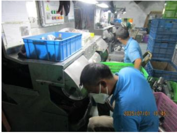
One employee working in polishing workshop contacted with noise did not wear earplugs which were provided by the facility.jpg One employee working in metalworking workshop contacted with noise did not wear earplugs which were provided by the facility.jpg
